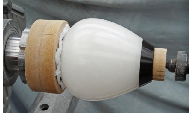
13. Finish shaping of the base
