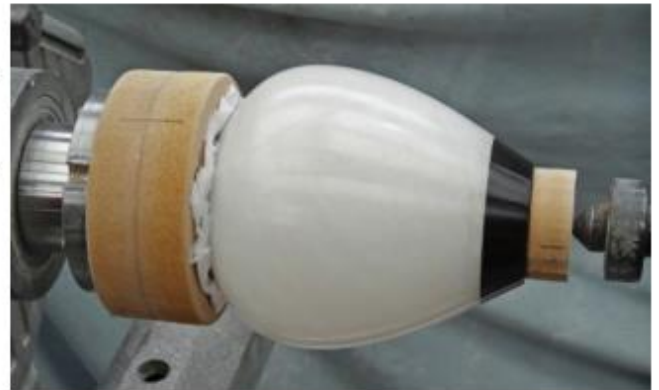
13. Finish shaping of the base
