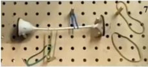
7 what he calls his 'torture rack', photo 7 : a pegboard with movable pegs and rubber bands to tension the wood to form curves in the stem.
